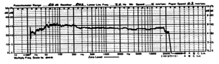
Spectral energy profile of an AR-90 in a typical listening room with the rear panel of the enclosure against the rear 15½-foot wall, its right woofer approximately 5 feet from the right-side wall and its left woofer approximately 9 feet from the left-side wall. Note the smooth response in the bass region and the absence of serious peaks and dips.
