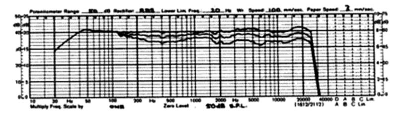
Effect of all the upper-range controls on the absolute acoustic output of the upper-range drivers when each control is set at "-0 dB", "-3 dB", and "-6 dB".
