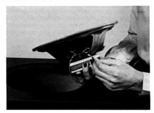
Replace the machine screws in the threads in the enclosure and finger tighten to prevent their loss.
