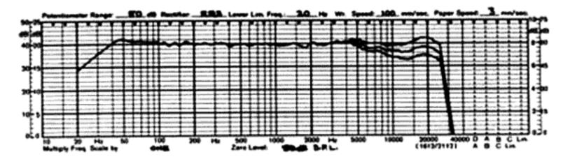
Effect of highrange control on the absolute acoustic output of highrange driver when it is set at "-0 dB", "-3 dB", and "-6 dB".
