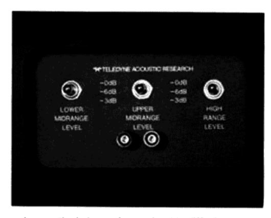
In most rooms and situations in which there is normal acoustical absorption and treble diffusion effected by drapes, shelves, bookcases, furniture, etc., and where associated equipment and source material of very high quality are being used, the switches should be placed in the "-0 dB" position.
