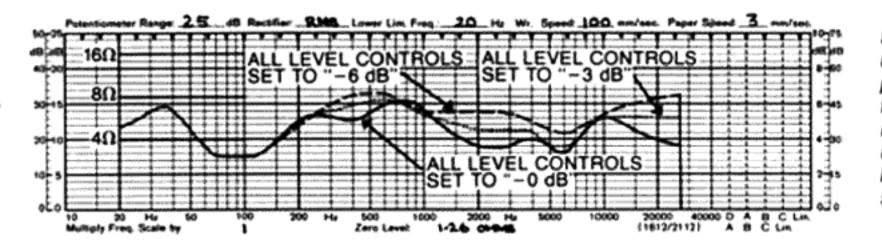
Logarithmic impedance plots of AR-90 for the three indicated upper-range level-control settings.
