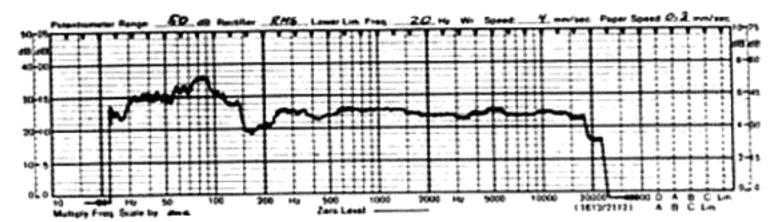
Spectral energy profile of a conventional speaker with a single, front-facing woofer in the same location (speaker catercornered) as the AR-90 above. Note the up-to-18-dB variations in the energy level and rough response extending from 40 Hz to 600 Hz.
