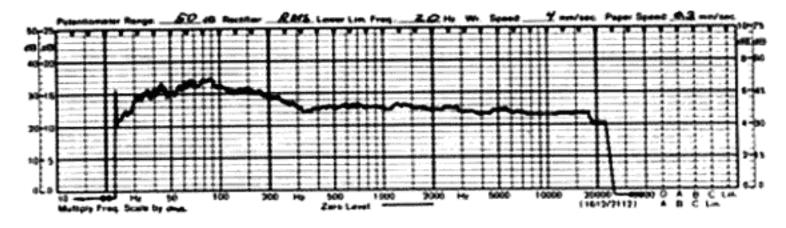
Spectral energy profile of an AR-90 in a typical listening room with the speaker catercornered and the rear panel at an angle to the rear 15½-foot wall.
