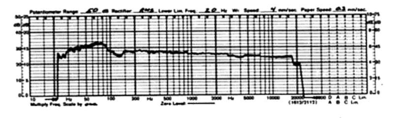
Spectral energy profile of an AR-90 in a typical listening room with the rear panel of the enclosure against the rear 15½-foot wall and its left woofer approximately 20 inches from the left-side wall.
