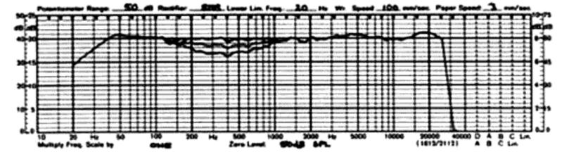
Effect of lowermidrange control on the absolute acoustic output of lower-midrange driver when it is set at "-0 dB", "-3 dB", and "-6 dB".
