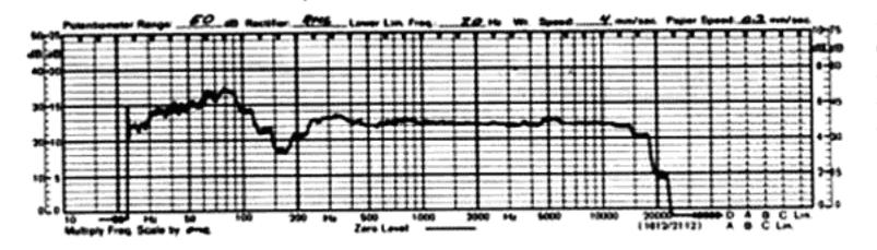
Spectral energy profile of a conventional speaker with a single, front-facing woofer in the same location (20 inches from the left-side wall) as the AR-90 above. Note the 20-dB peak-to-trough ratio in the energy level between 50 Hz and 200 Hz which is minimal in the AR-90 profile.
